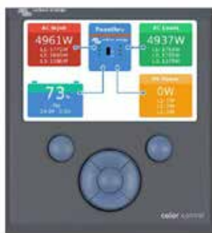
Color Control GX, showing a PV application
