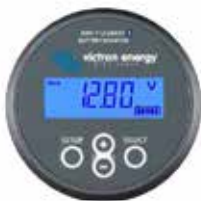
Bluetooth sensing: BMV-712 Smart Battery Monitor
