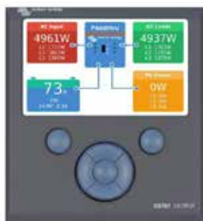
Color Control GX, showing a PV application
